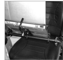
Adjustable tilt with quick release lever
