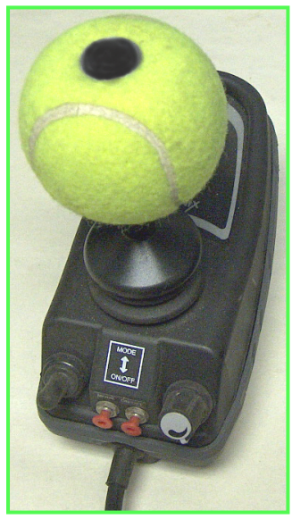
The Interchangeable Knob Interface allows your client to easily customize their chair with "off the shelf" hardware store knobs.
