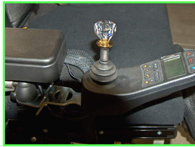
The Interchangeable Knob Interface allows your client to easily customize their chair with "off the shelf" hardware store knobs.
